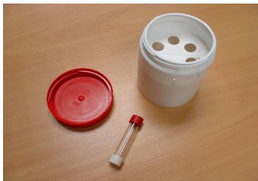
Tube passif NO 2 et support (Source : ATMO Grand Est)
