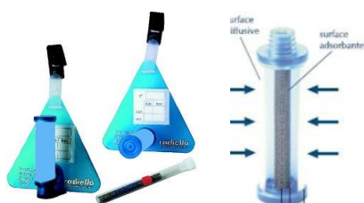
Figure 3 : Tubes passifs radiello
