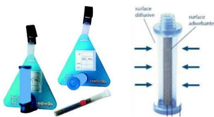
Figure 3 : Tubes passifs Radiello
